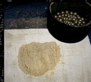
6. Remove steel balls from the milled powder
