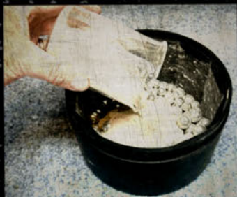
4. Process crushed uranium using a ball mill
